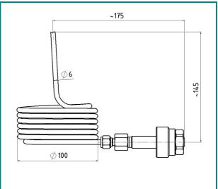
Connecting spirals in stainless steel 1.4404 are the connecting tubes between gas cylinders and gas supply stations. The connecting spirals are fitted with a hand nut and gas specific connections to DIN477 und CEN-Hevos.
